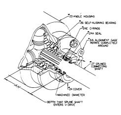
to the joint end that is on the spool adapter. This distance will not with misalignment vary since the joint is bolted and cannot move.) Put the #31A alignment gauge on the machined diameter of the #24 cover and slide it completely around. It will indicate how the engine must be moved to center the spline shaft in the oil seal. Re-measure joints see if the to
