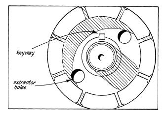
(c) With a suitable nylon drift and hammer, gently tap the injection pump shaft to dislodge it from the keyed drive gear. The loose hold down nuts will prevent the pump from falling from the engine.
