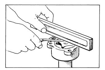
4. Then, place a straight edge across the pump cover and measure the clearance between the straight edge and cover. If the cover exceeds the limit, correct the pump cover by grinding or replace it.
