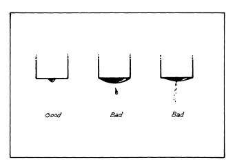
3. Checking Oil Tightness of Needle Valve Set
