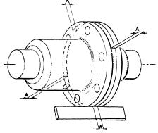
90° between each position. This test will also check whether the propeller half coupling is in exact alignment on its shaft. Then, keeping the propeller coupling in one position, the alignment should be checked rotating the engine half coupling to full position each 90° from the next one.
