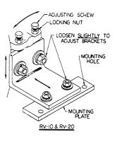
tighten the nuts. Place the V-drive on the engine bed, lining it up "by eye" to the propeller shaft flange as closely as possible. Firmly bolt it down through the holes provided in the mounting plates. Loosen the locking nuts on the adjusting screws. Slightly loosen the nuts on the mounting brackets just enough to be able to move the Vdrive.
