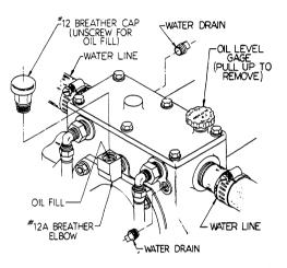
Additional Molykote after break-in is not required. Reinstall the breather cap. The oil level should be rechecked after the unit has been run and allowed to sit for about a minute. Add oil if necessary.
