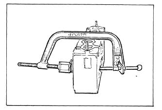
NOTE: After removing the value assemblies, arrange or label them in the order of removal so that they can be reinstalled in their original positions.
