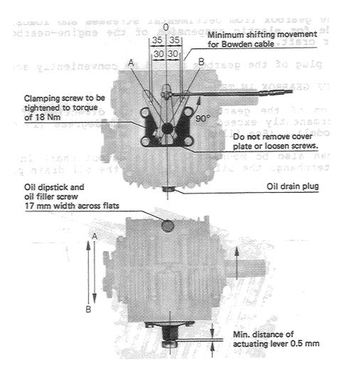
The position of the cover plate underneath the actuating lever is factory-adjusted to ensure equal lever travel from neutral position to A and B. Therefore, do not loosen the capscrews mounting this assembly. Removal or disturbing of the shift cover will void all warranty responsibilities by Westerbeke.
