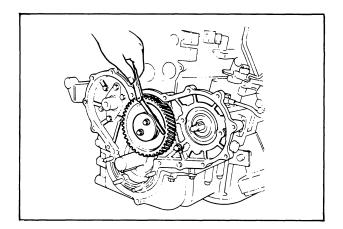
Thrust plate tightening torque: 2.3 - 3.2 kg-m (17 - 23 lb-ft)
