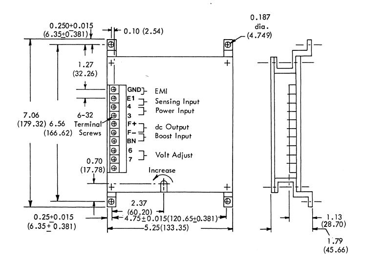
Note: Numbers in parentheses are in millimeters. Tolerance <u>+</u> 0.03 (0.762) unless otherwise noted.
