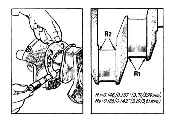
NOTE: Measure the diameter of each of the crankpins and main journals at two points (the front and rear portions) at 90 degrees to the crankshaft axis, as shown in figure.
