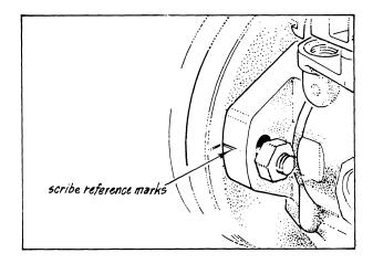
(a) Loosen the two injection pump hold down nuts. Do not remove entirely. The hold down nut on the engine side of the pump can be gotten at by using a 1/4" universal socket and extension with ratchet.
