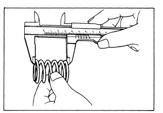
Check the squareness of valve spring. If it exceeds the limit, replace with a new one.
