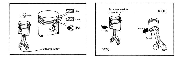
4. Piston rings. Use a suitable piston ring expander.
