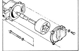
Cover tightening torque: 0.8 - 1.2 kg-m (5.8 - 8.7 lb-ft)
