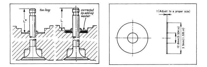
When the dimension "L" becomes more than 1.5 mm (0.059 in) larger than the standard, replace both the valve and cylinder head.
