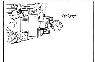
NOTE: When setting the dial gauge, confirm that the dial gauge pointer does not deviate from the scale mark of zero by slightly turning the engine crankshaft from left to right.
