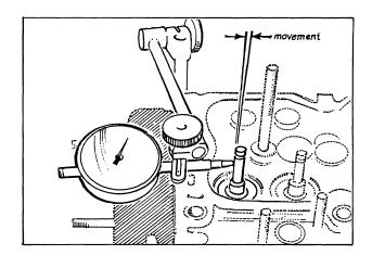
Check the protruding length of the valve guide. If it is not the specification, correct it.
